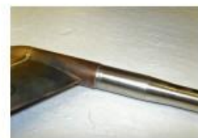
Probe for a CRJ jet made of beryllium copper and nickel
