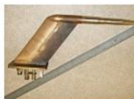
Probe for a CRJ jet made of beryllium copper and nickel
